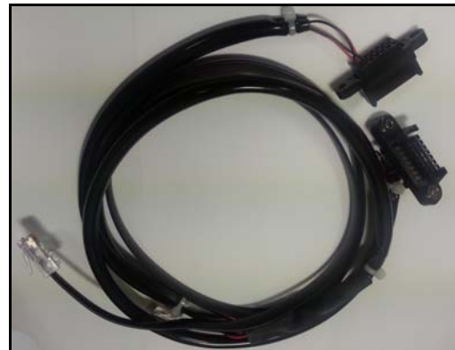
Figure 3: JCM BlueWave Adapter Cable (P/N 400-000086R)
