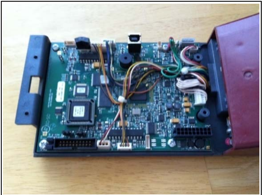
Figure 11 One-Time Programmable (OTP) CPU
